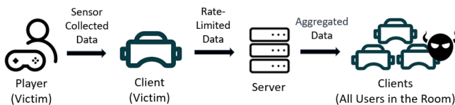
Figure 2: Motion data flow in multi-user VR applications.
